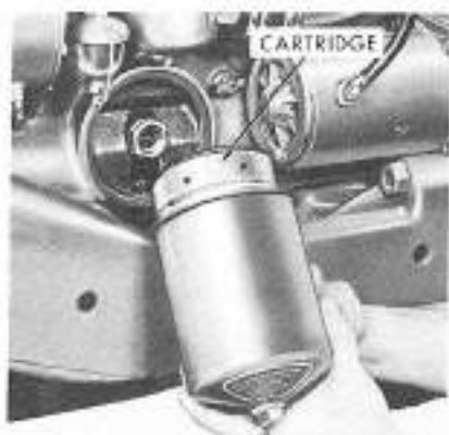
Figure 27 Replacing the Oil Filter Cartridge
