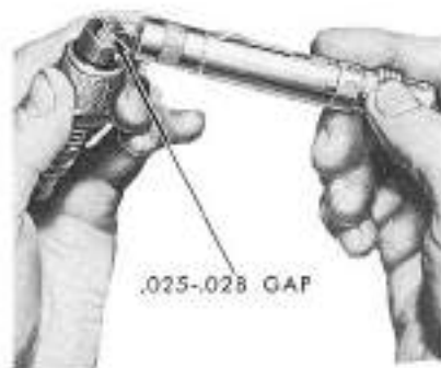
Figure 36 Checking Spark Plug Gap
