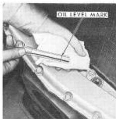
Figure 25 Checking Pedestal Oil Level
