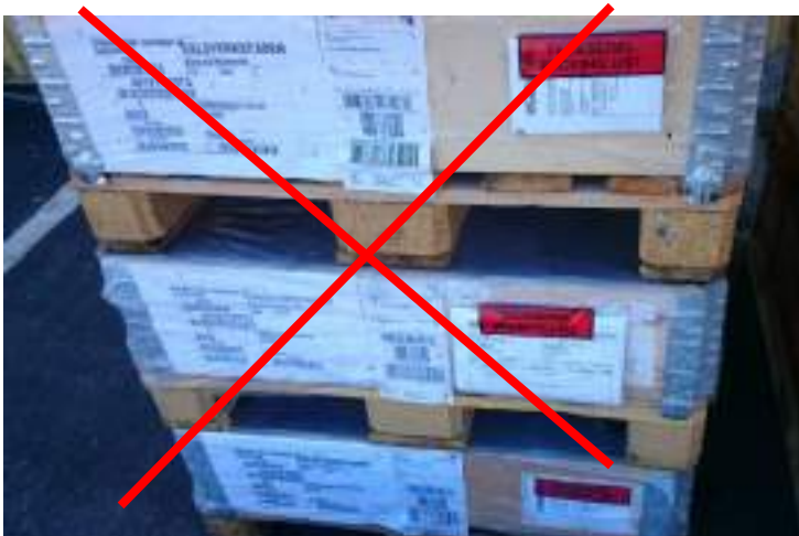
Figure 30G Stacked pallets but only plastic fill in between
