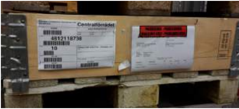
Figure 29 Packing label attached to the pallet, in a plastic envelope beside the odette label
