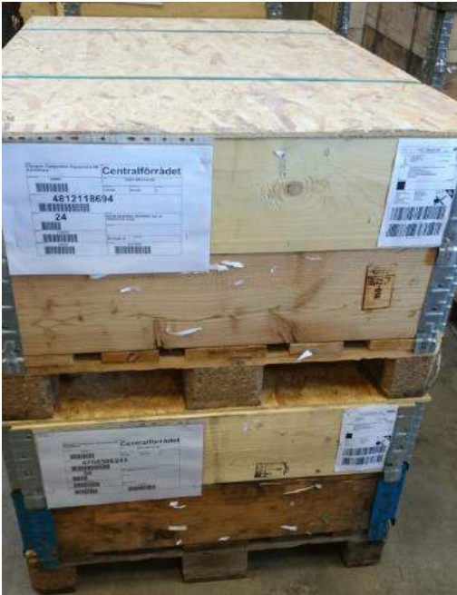
Figure 30E Pallets correctly stacked, with lids in between
