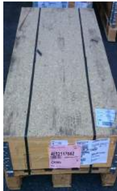
Figure 30H Cover the open pallets with a lid
