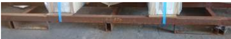
Figure 28 A and B: the fork tunnels in the right direction to enable unloading
