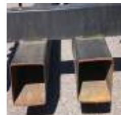
Figure 28 A and B: the fork tunnels in the right direction to enable unloading
