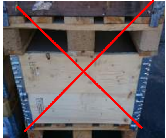
Figure 30F Stacked pallets but with out lids in between
