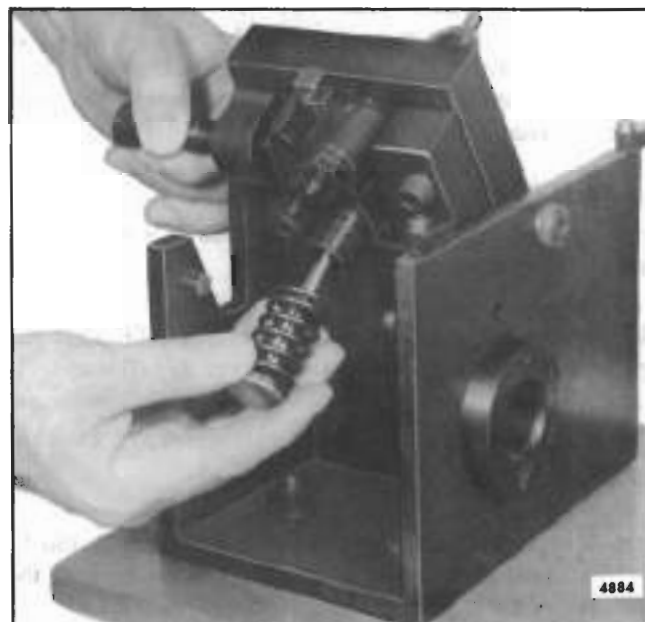
Fig. 24 - Removing or Installing Plunger Follower, Plunger and Spring
