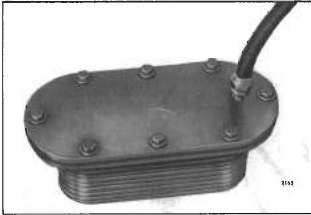
Fig. 6 - Oil Cooler Core Prepared for Pressure Check
