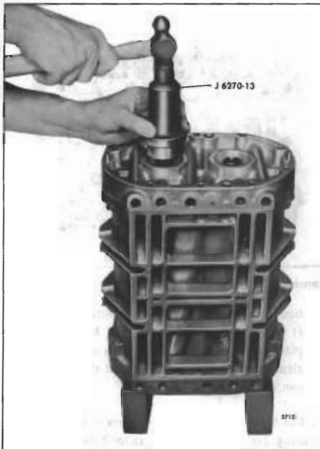
Fig. 17 - Installing Roller Bearings on Rotor Shafts and in Front End Plate
