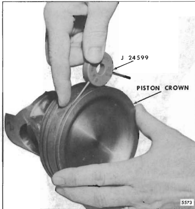
Fig. 5 - Checking Fire Ring Groove in Piston Crown
