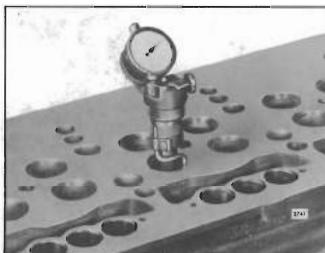
Fig. 14 - Checking Relative Concentricity of Valve Seat Insert with Relation to Valve Guide
