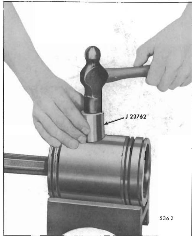
Fig. 9 - Installing Piston Pin Retainer
