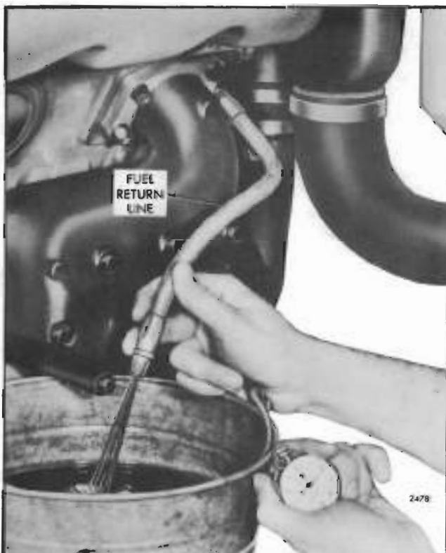
Fig. 7 - Measuring Fuel Flow From Fuel Return Manifold
