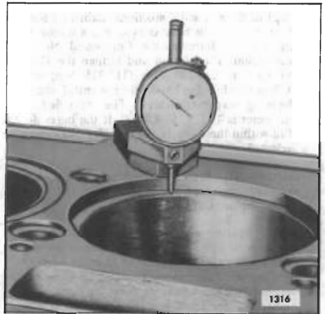
Fig. 5 - Checking Depth of Counterbore with Tool J 22273
