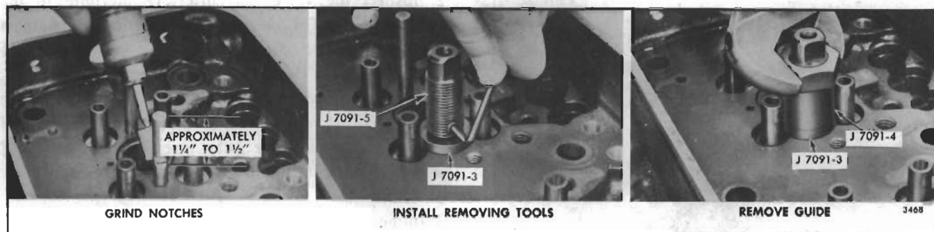
Fig. 8 - Removing Press-Fit Exhaust Valve Bridge Guide
