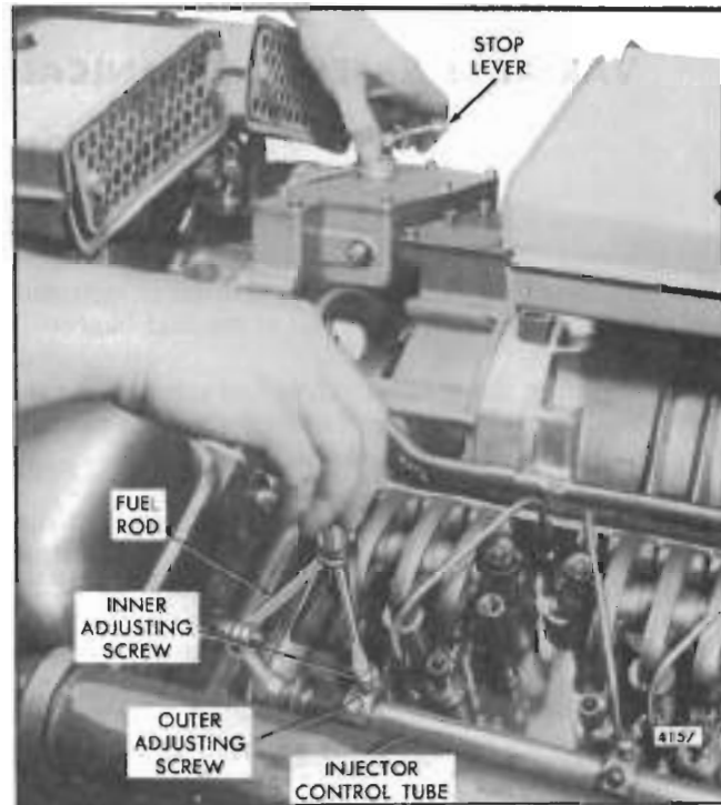
Fig. 4 - Positioning No. 4R Injector Rack Control Lever
