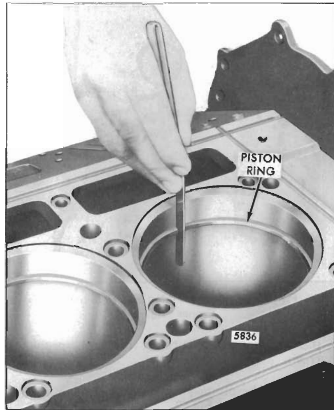
Fig. 14 - Measuring Piston Ring Gap
