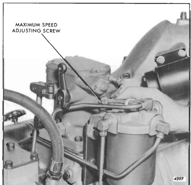
Fig. 11 - Adjusting Maximum No-Load Engine Speed
