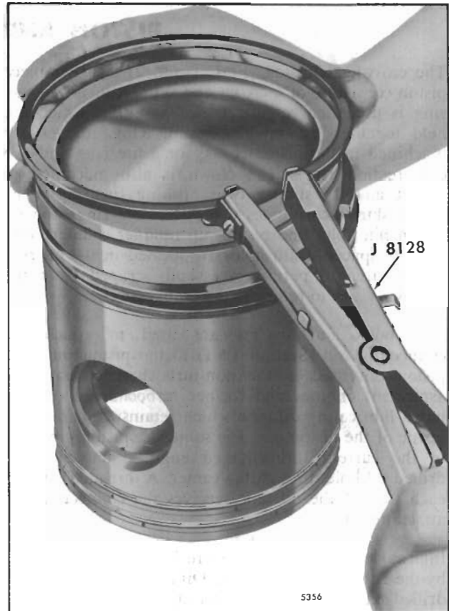
Fig. 4 - Removing or Installing Piston Rings
