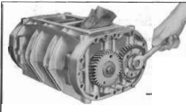
Fig. 18 - Installing Blower Rotor Timing Gears
