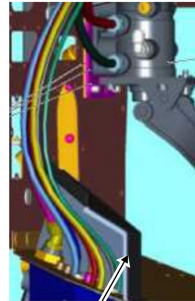
Airlines and cab pass through are located under the drivers dead pedal
