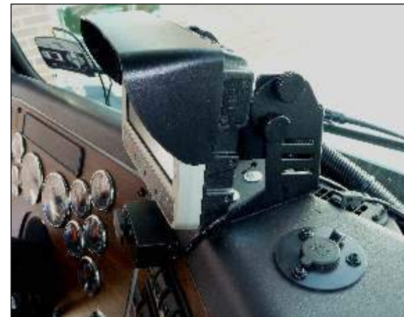
AWTI Camera Mounted using common mounting pattern
