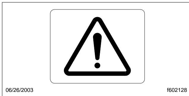
Fig. 2.29, Roll Stability Indicator Lamp
