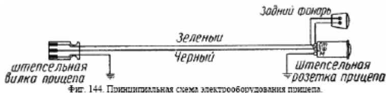
Fig. 144. Schematic diagram of the electrical trailer.
