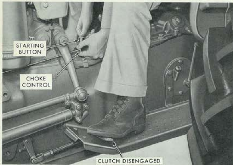
Figure 11 Using the Starter Button, Choke and Clutch Pedal
